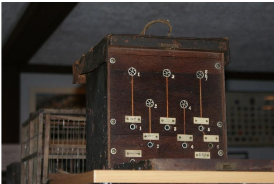
Switchboard to the 38 th Battalion CEF, 4 Canadian Divisional Signals
